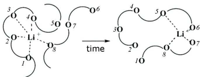
*Schematic diagram of lithium ion conduction mechanism of PEO-based polymer electrolyte. [Reproduction with permission from Xu (2004), Copyright 2004, American Chemical Society].*
